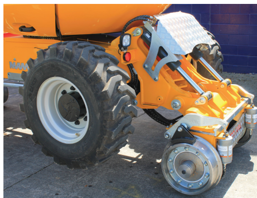
Additional spring applied, hydraulic release fail-safe brakes on all wheels, additional to independent fail-safe parking brakes
